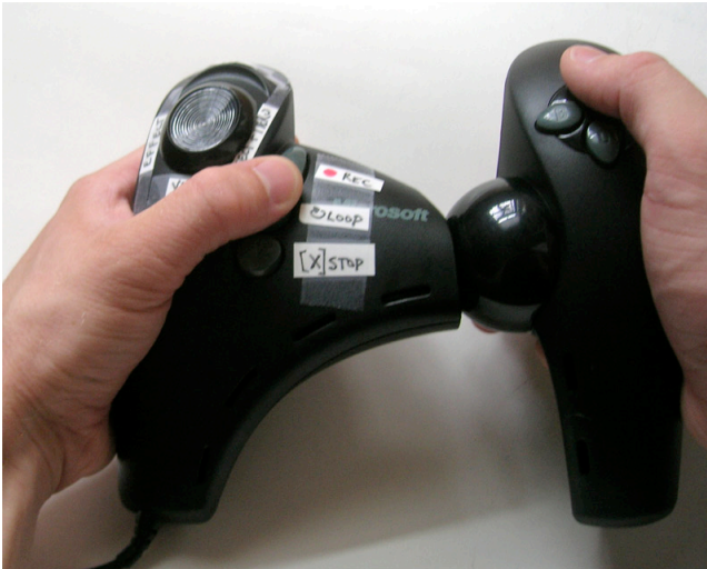
Figure 2: The joystick interface used for the PureJoy instrument. A PureJoy player also wears a headset/mic that allows for personalized auditory instructions, and vocal or other sonic input.
